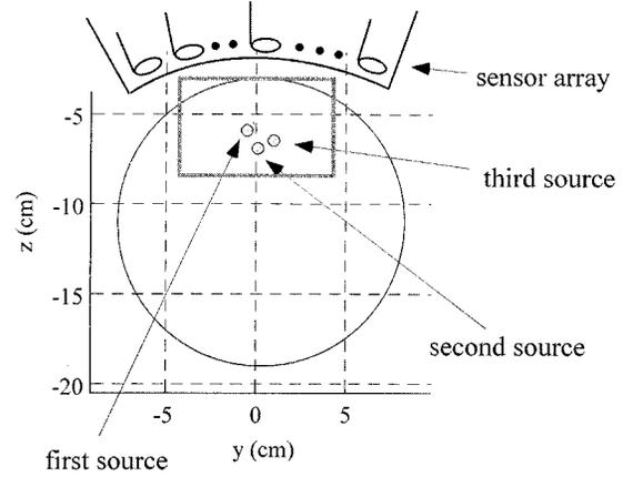
Fig. 1. The coordinate system and the source-detector configuration used in the numerical experiments. The coordinate origin was set at the center of the detector coil located at the center of the coil array. The cross section at  $x = 1.0$  is shown. The circle shows the cross section of the sphere used for the forward calculation. The square shows the reconstruction region for the experiments whose results are shown in Figs. 3–6.
