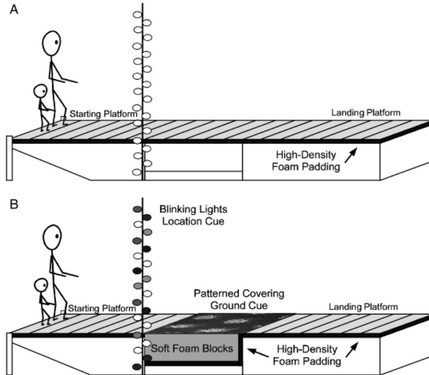
Figure 1. Configuration of walkway and foam pit. (A) The walkway remained continuously solid during baseline trials, (B) but was interrupted by a deformable foam pit in the test trials. The foam pit was always marked by the patterned ground covering and blinking colored lights landmark. The stick figures represent approximately scaled sizes of infant and adult participants.
